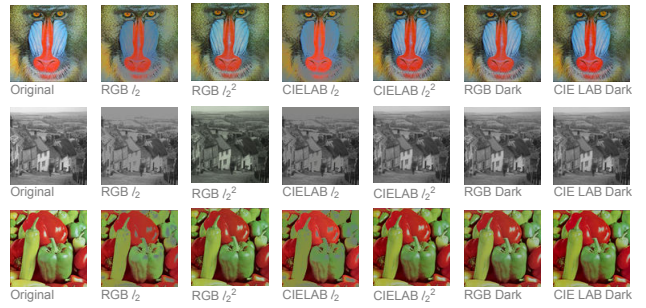
Figure 10. Effect of color transforms all configured to cause a 25% reduction in display power dissipation.
